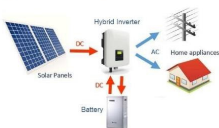
Typical Power Flow in Solar Hybrid Solutions
